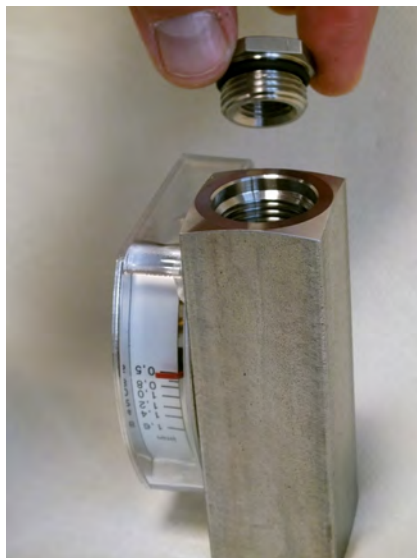
Fig. 53: Insert process connection (inlet)
