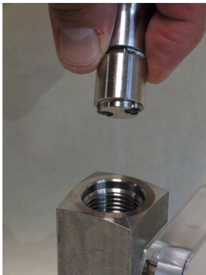
Fig. 44: Insert threaded ring insertion tool (outlet)
