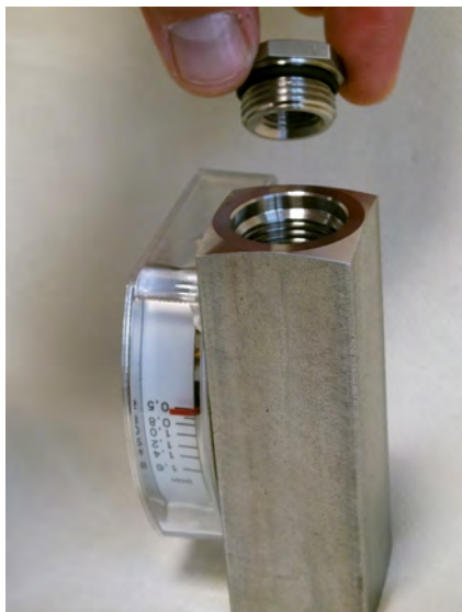
Fig. 50: Remove the process connection (inlet)
