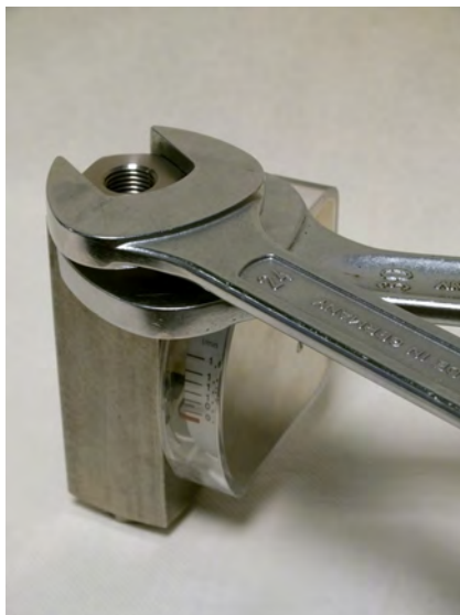
Fig. 42: Loosen process connection (outlet)
