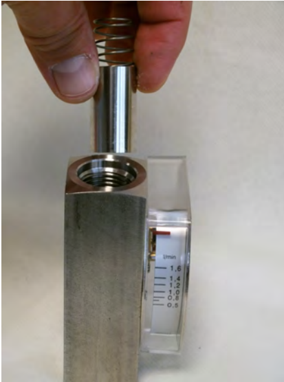
Fig. 56: Insert inner parts
