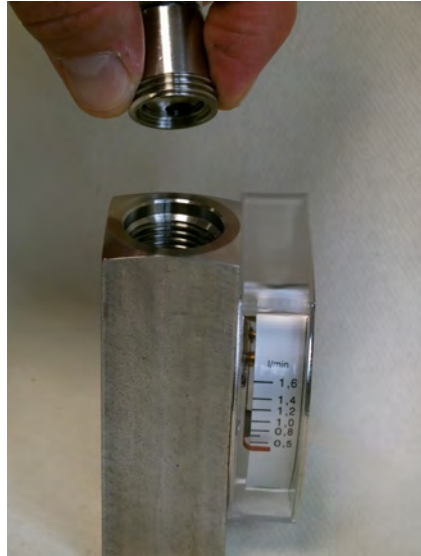
Fig. 46: Remove threaded ring (outlet)
