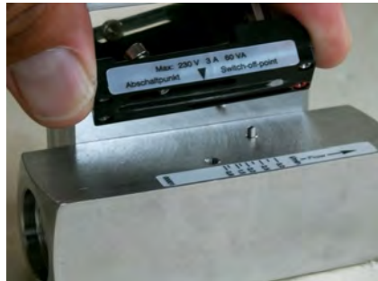
Fig. 70: Remove switch contact
