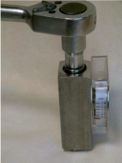
Fig. 45: Loosen threaded ring (outlet)
