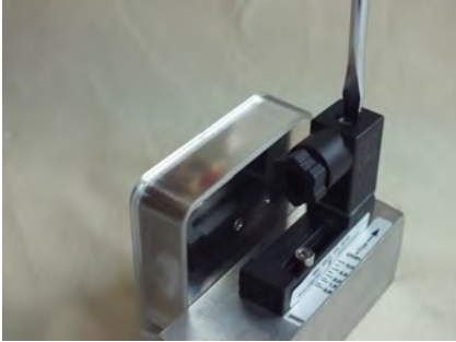
Fig. 67: Loosen female socket
