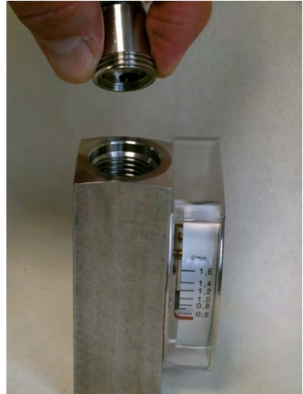
Fig. 57: Insert threaded ring (outlet)
