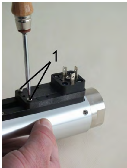
Fig. 55: Loosen set screws
