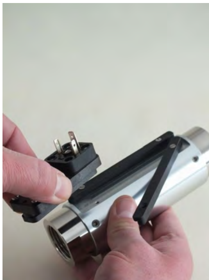
Fig. 58: Remove switch contact
