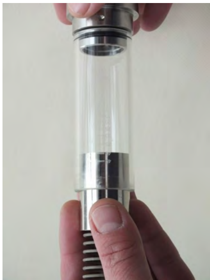
Fig. 39: Remove float and spring
