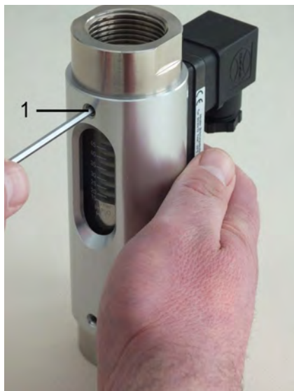
Fig. 36: Remove the process connection (outlet)
