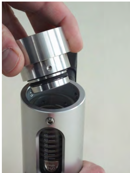
Fig. 36: Remove the process connection (outlet)
