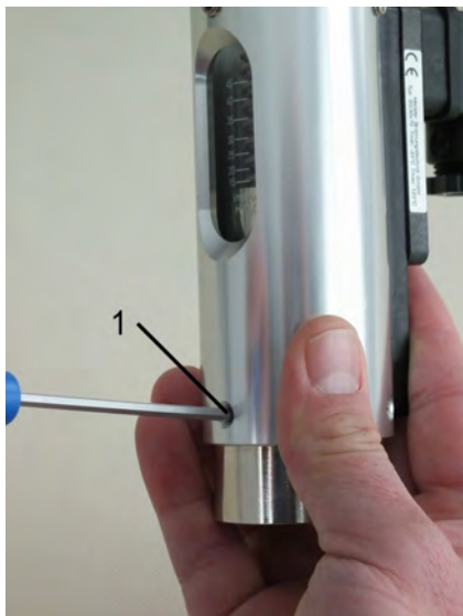
Fig. 47: Secure the process connection (inlet)
