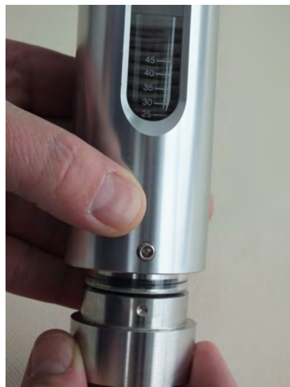
Fig. 46: Insert the process connection into the device housing
