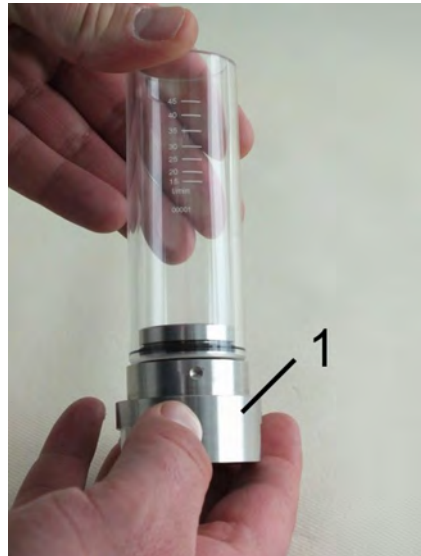
Fig. 44: Process connection (inlet) and sight glass
