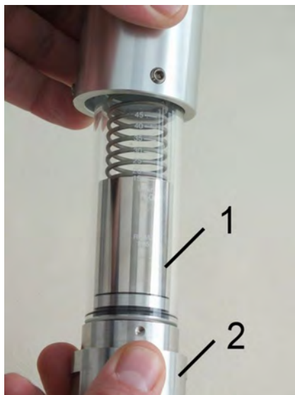
Fig. 38: Remove the inner parts
