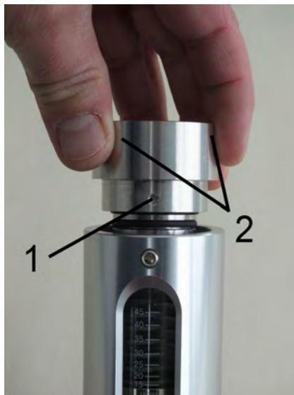
Fig. 50: Position the process connection (outlet)
