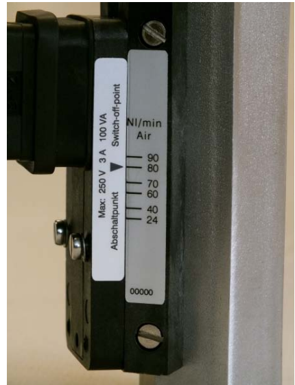
Fig. 4: Switch point adjustment scale RVM/U-L2 30x70
