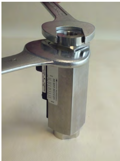
Fig. 58: Tighten process connection (outlet)
