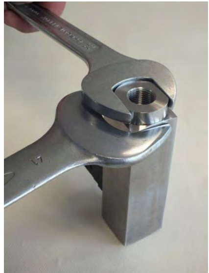
Fig. 42: Loosen process connection (inlet)
