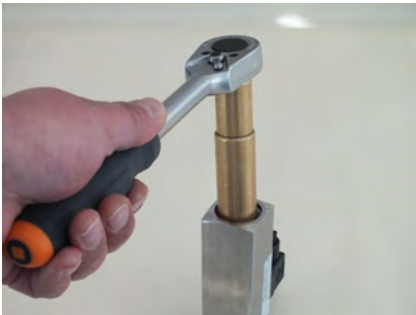
Fig. 50: Seat threaded ring (inlet)
