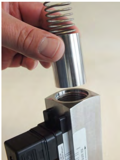
Fig. 54: Insert inner parts
