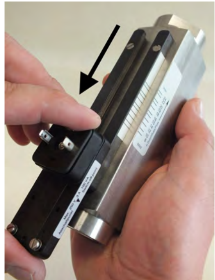
Fig. 63: Remove switch contact from guide rails
