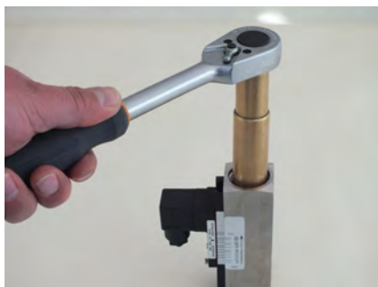
Fig. 38: Loosen threaded ring (outlet)
