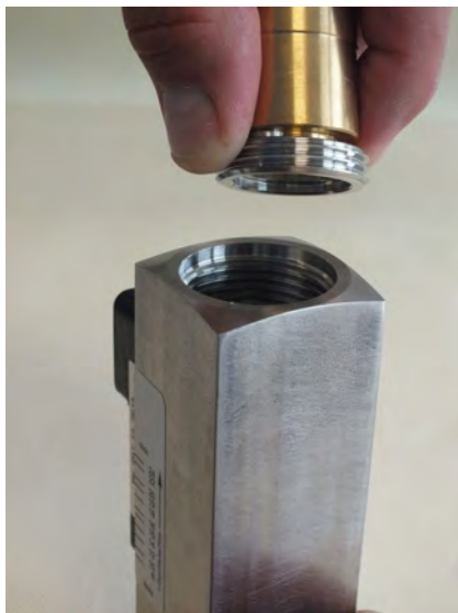
Fig. 55: Insert threaded ring (outlet)
