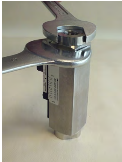
Fig. 35: Loosen process connection (outlet)
