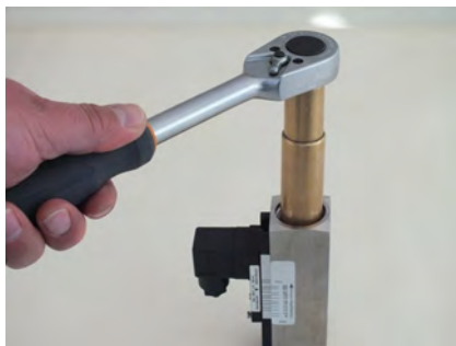
Fig. 56: Seat threaded ring (outlet)
