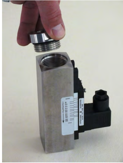
Fig. 51: Remove the process connection (inlet)
